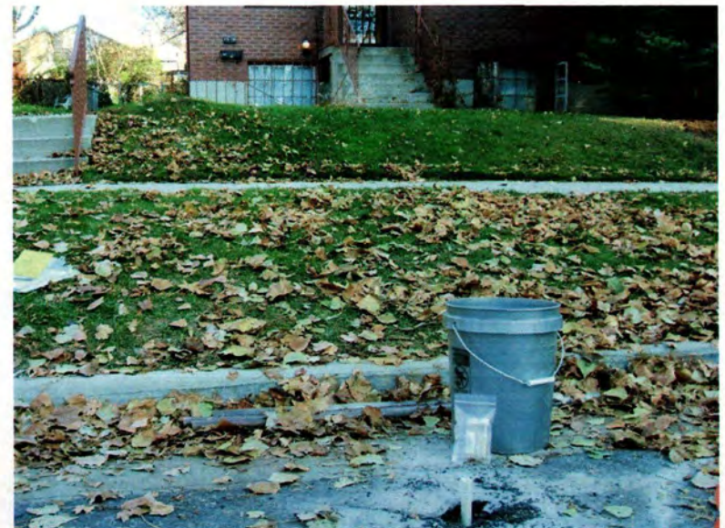
East Side Springs View: East 11/15/11 ESS-GW-10. Collected groundwater sample ESS-GW-10. Returned to the location to find 5.5 feet of water in the temporary PVC well.
