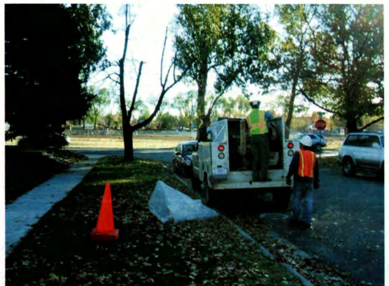
East Side Springs View: South 11/14/11 URS setting up the direct-push unit at sample location ESS-GW-10 (1259 South Lake Street). Direct-push unit would breakdown at this location.
