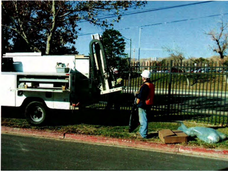
East Side Springs View: North 11/16/11 URS setting up the direct-push unit at soil-gas location ESS-SG-31. Sample located just east of the main Hospital entrance along 500 South.
