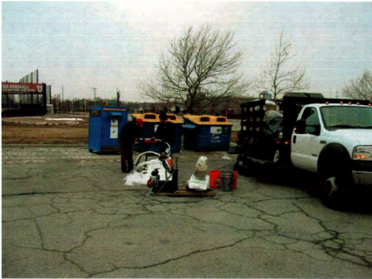
East Side Springs View: South 12/21/11 URS setting up the inertia pump at monitoring well EPA-MW-01D. Well is located in the southwest corner of the SLC Sports Complex parking area.
