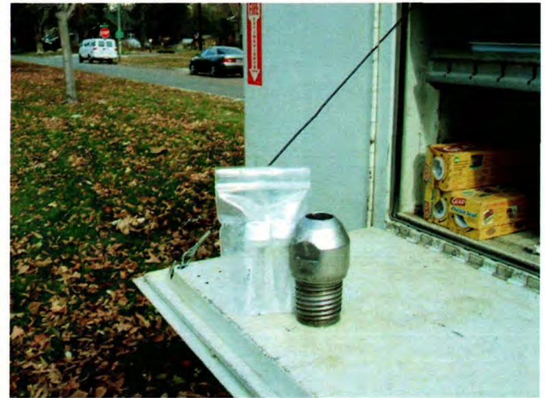
East Side Springs View: N/A 11/15/11 ESS-GW-13. Collected rinsate blank sample ESS-GW-13. Photo of sample with the decontaminated direct-push shoe.
