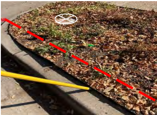
Metal landscaping rings potentially interfering with magnetometer readings near MW-61.
