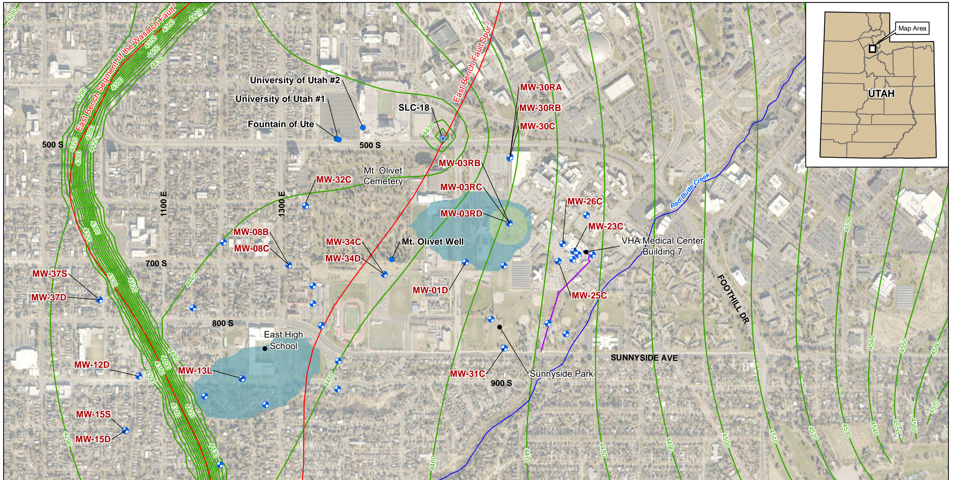
Figure 4-21a Future Conditions - Initial PCE Concentrations Deep Aquifer Scenario 4: Proposed University Irrigation Pumping and Maximum (Water Right) Pumping at SLC-18
