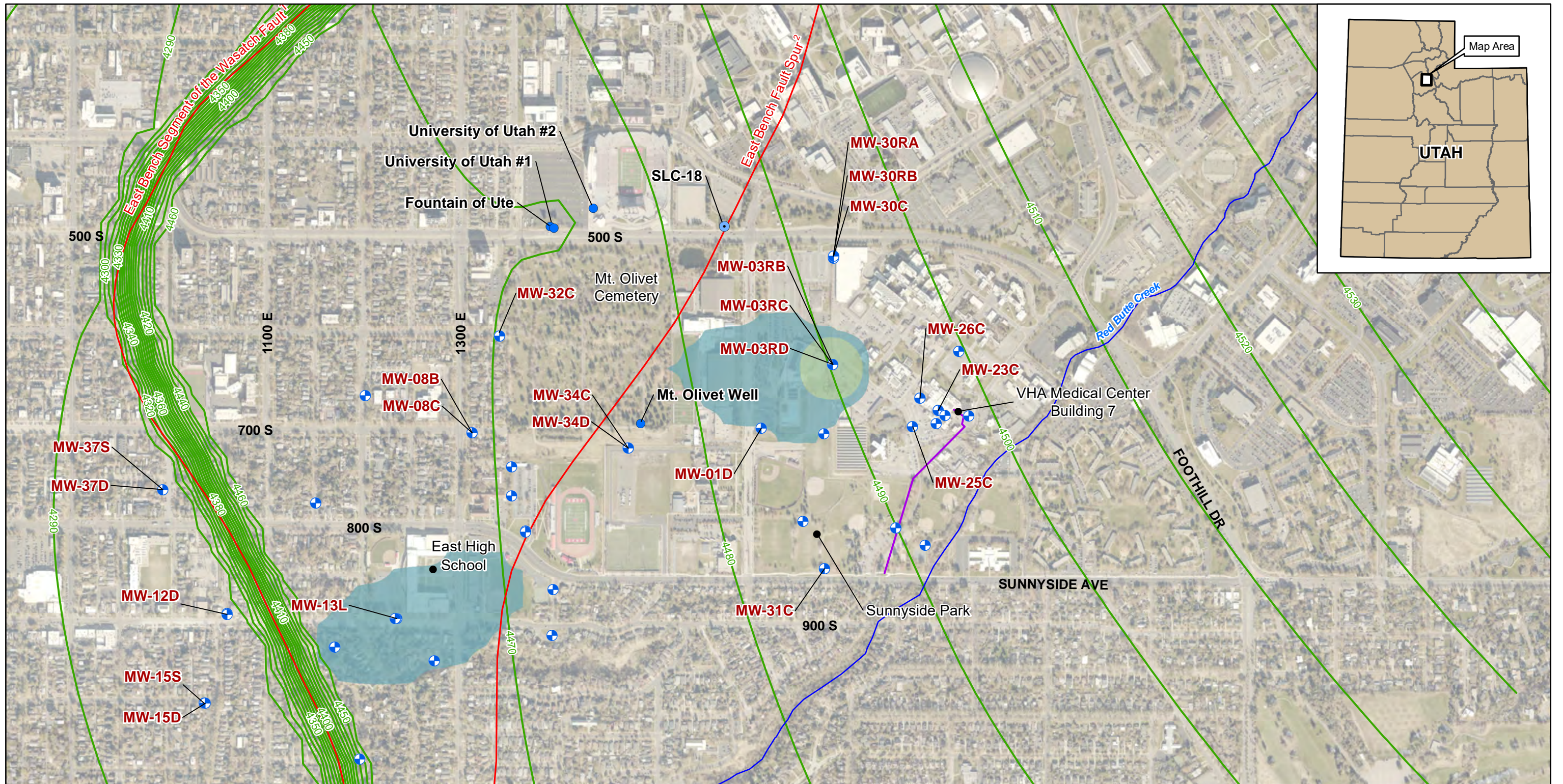
Figure 4-19a Future Conditions - Initial PCE Concentrations Deep Aquifer Scenario 3: Proposed University Irrigation Pumping
