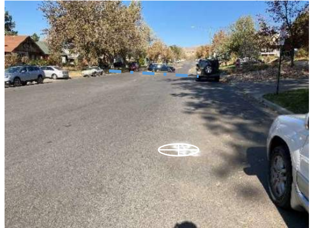
MW 38 (1200 E option) Water located along sidewalk and crossing the street to the North of the proposed location. Recommend engaging Blue Stake before proceeding.
