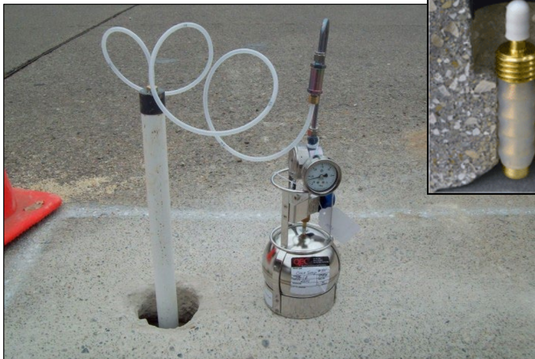
Soil Gas Probe Sample Collection
